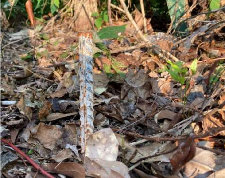
*Figure 3 Iron pins like this one often mark property boundaries. These are key to identifying lot lines. Other markers include pipes, pieces of metal, or stakes with bright flagging on them.*
